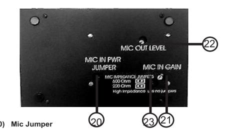
Plugging the jumper (shorting block) puts +5V on the Mic In line of the microphone's cartridge (11, 12 & 13). Required for mic's such as ICOM's Hm12, HM36 and Sm6 and the Heil Hmi and MH2 (made for the Elecraft radio's) and other electret microphones.
