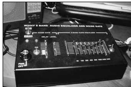
Figure 1 — W2IHY 8 Band Audio Equalizer and Noise Gate
